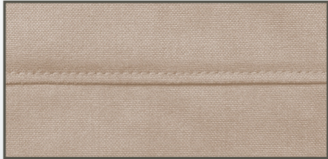
2 French Seam/ Single Needle
