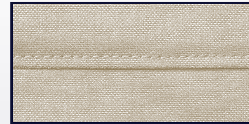
2 French Seam/Single Needle
