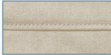
2 French Seam/ Single Needle
